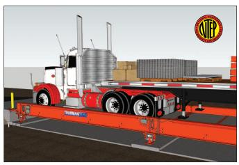
Thurman Scale's 8530KD is a fully electronic, side rail scale designed for easy field assembly and on-site concrete deck pour. This scale is a popular choice for weighing wide fertilizer trucks and other oversize farm vehicles.
