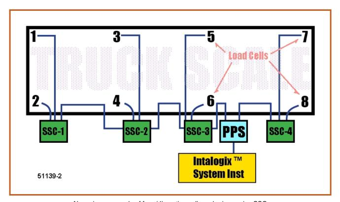
Above is an example of four (4) section cell numberings using SSCs.
