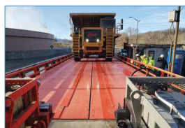
Custom 8565 truck scale with 80' x 20' deck and 400,000 pound capacity.
